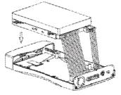
9. Secure the cradle with the four retaining screws.
